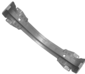
684.440 = TRAVESSA DO CHASSI E MOTOR MWM F-11000 / F-12000 / F-13000
